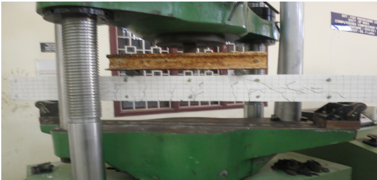
Figure (4): Shear cracks in preloaded SD beam prior to repair
