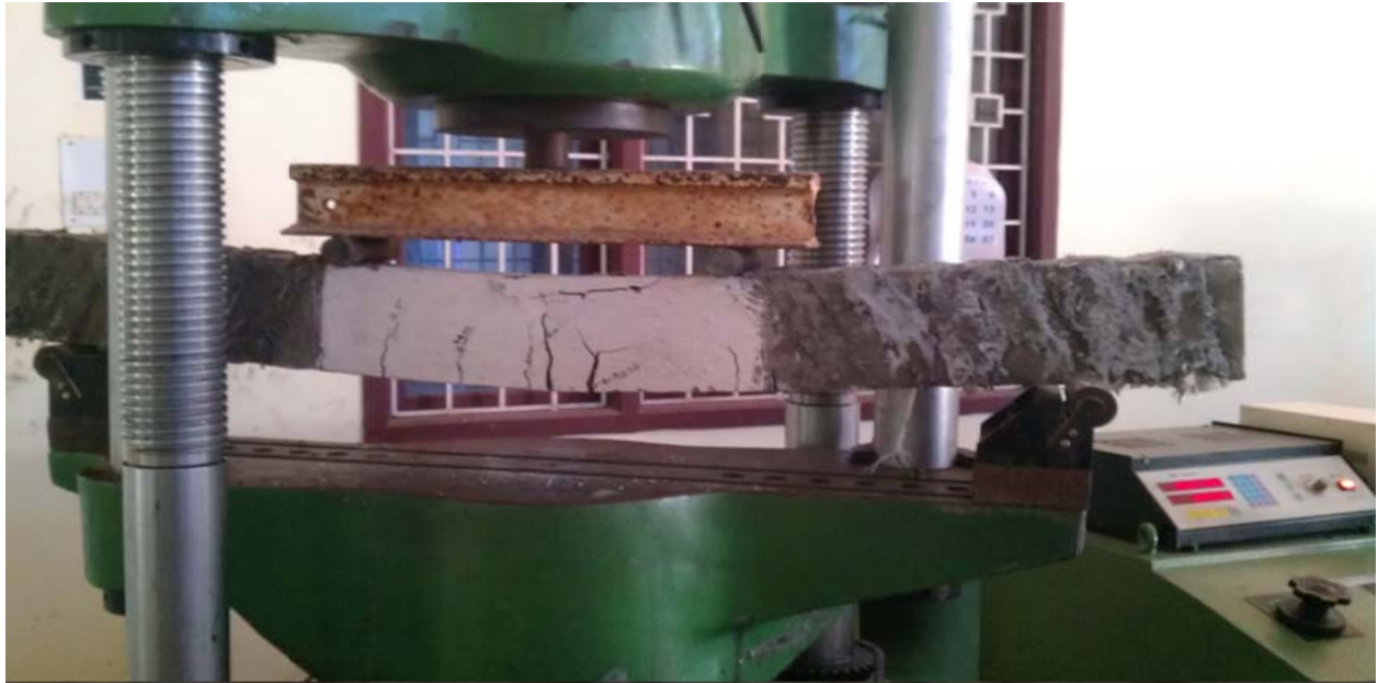
Figure (6): Retrofitted damaged RSD beam loaded to failure
