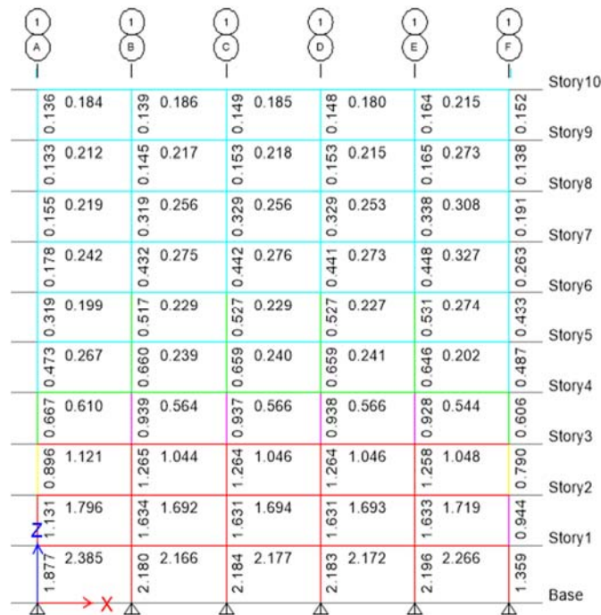
Figure (7b): Demand/capacity ratio for load combination (1.2D + 1.0L + 1.0W) stability analysis using ELM
