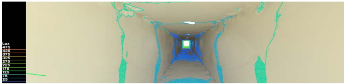
Figure (14): The illuminance environment in the corridor with light pipes at 2 pm
