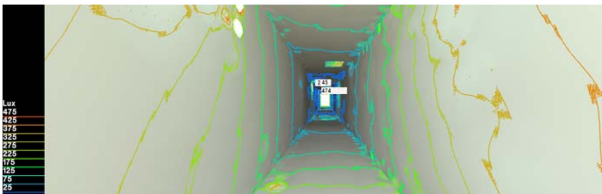
Figure (10): The illuminance environment in the corridor with an anidolic system at 8 am
