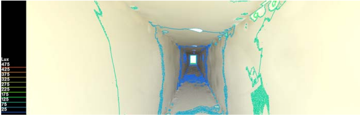
Figure (11): The illuminance environment in the corridor with light pipes at 8 am
