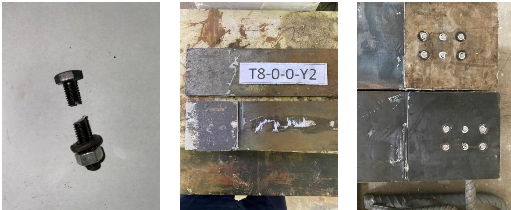
Figure (5): Failure in bolts, glued plates and glued plates with bolts
