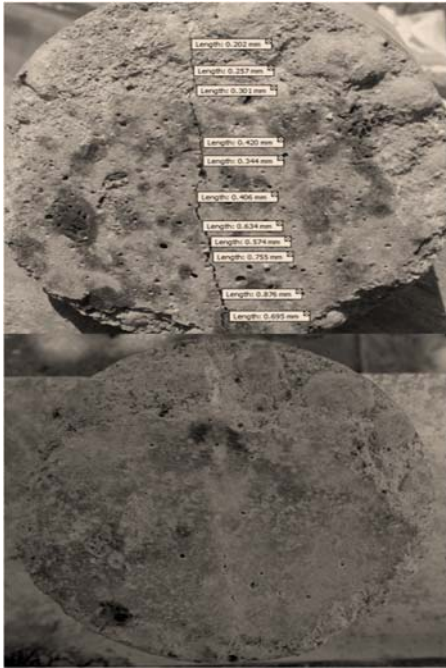
Figure (5): Crack widths of light-weight bacterial concrete before and after 56 days of healing
