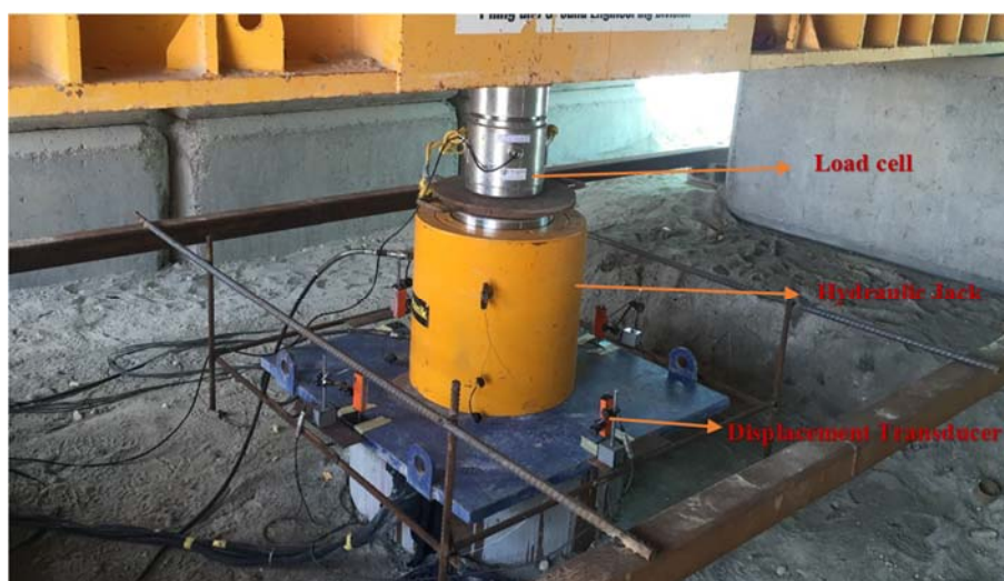
Picture (2): CFA pile test setup
