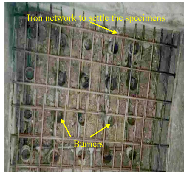
Figure (3): Brick stove of net methane burner
