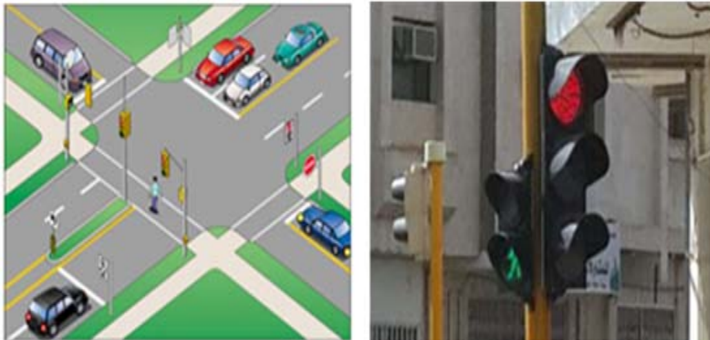
Figure (3): Pedestrian crossing signals at intersections
