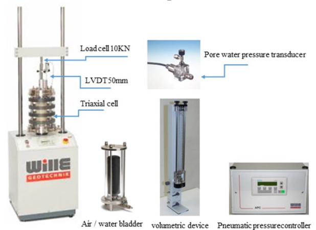
Figure (5): An overall view of the cyclic triaxial system
